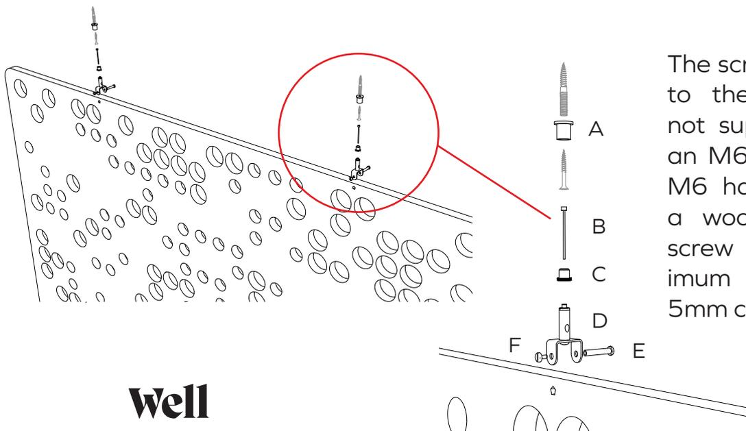
The screws for fixing to the ceiling are not supplied. Either an M6 set screw, a M6 hanger bolt or a wood chipboard screw with a maximum diameter of 5mm can be used.
