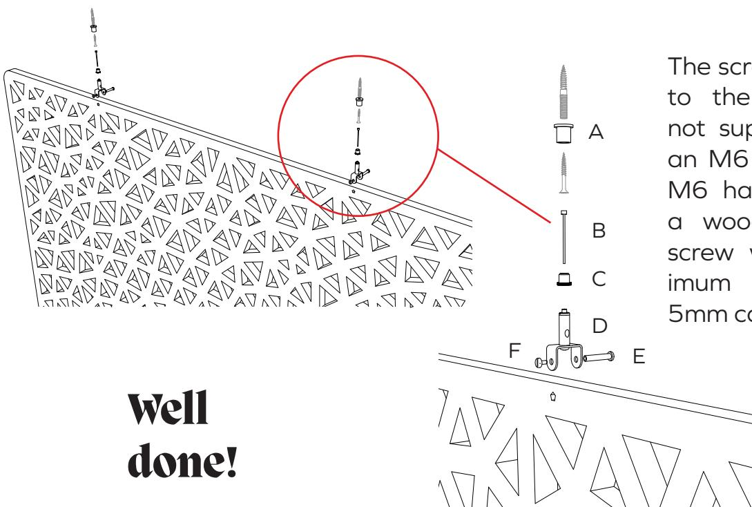
The screws for fixing to the ceiling are not supplied. Either an M6 set screw, a M6 hanger bolt or a wood chipboard screw with a maximum diameter of 5mm can be used.
