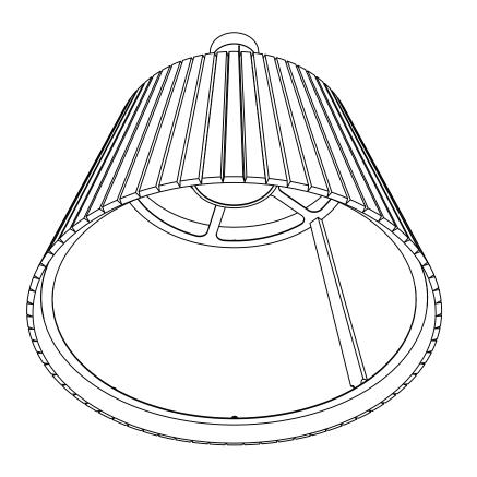
1. For Spark 1200 and Spark 1600 assembly, skip this step. Insert the luminaire body through the luminaire shade as shown.
